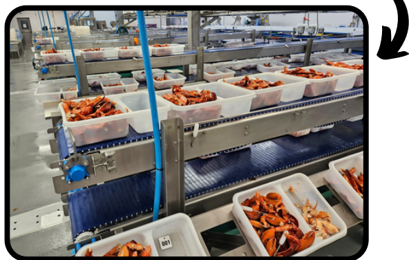
Double conveyor for Seafood sorting tables
